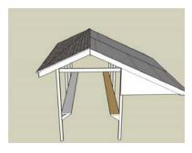
the GP range. The long baffle (overhang) to the right is approximately six feet from the grade and will be made up of a sandwich of plywood and steel. As you might imagine from the distance from the firing line to the baffle edge, you will not be able to fire above the top of the berm unless you are lying prone on the ground. This could be
